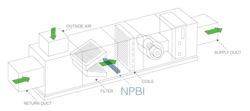
Inactivate pathogens | Break apart odors | Clump small particles together to filter out
