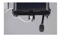
Attach the Stylus: The stylus should be attached into the headphone jack at the top right of the tablet.
