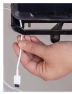
Secure Tablet Charger: Secure the tabletcharging cable by pushing down on the top and bottom of the case to close it. Be sure to plug the cable into the tablet with enough slack so as to not strain the cable at point of connection.
