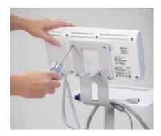
Remove Monitor from Stand: Once screws are removed, lift the Welch Allyn Vital Signs Monitor off the rolling-stand mount and set aside.
