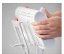
Attach the DS smart Mounting Plate with Attached Tablet to the Stand: Place the DS smart mounting plate with the attached tablet on the Welch Allyn stand mounting pegs. Stabilize the DS smart mounting plate with the attached tablet until it is secured in the next step.
