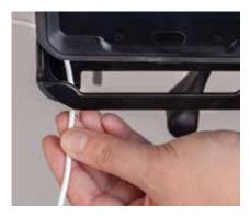
Secure Tablet Charger: Secure the tablet-charging cable by pushing down on the top and bottom of the case to close it. Be sure to plug the cable into the tablet with enough slack so as to not strain the cable at point of connection.
