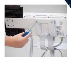
5 Attach the Power Strip to the Stand: Attach the power strip to the stem of the rolling stand by tightening the screw clamps.
