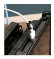
Attach the Stylus: The stylus should be attached into the headphone jack at the top right of the tablet.
