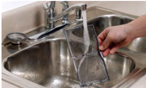
Step 5. Rinse the filter with running water and allow it to dry completely.
