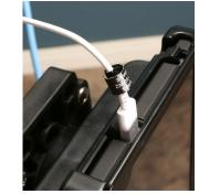
Attach the Stylus: The stylus should be attached into the headphone jack at the top right of the tablet.
