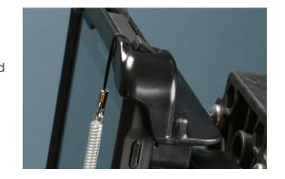
Attaching Cord Clips: Secure the white tablet USB cable to stand pole using the three clips as shown. Note that the clips arrive with the vital signs monitor stand.
